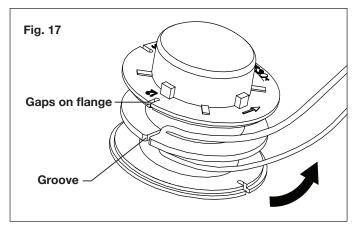
**3.** Wind both ends into the grooves using slight tension and following the direction of the arrows (Fig. 18).
